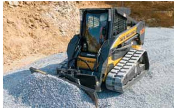
The see-through area on the cab roof provides a clear view to the bucket or attachment, even when it's positioned at full height.
