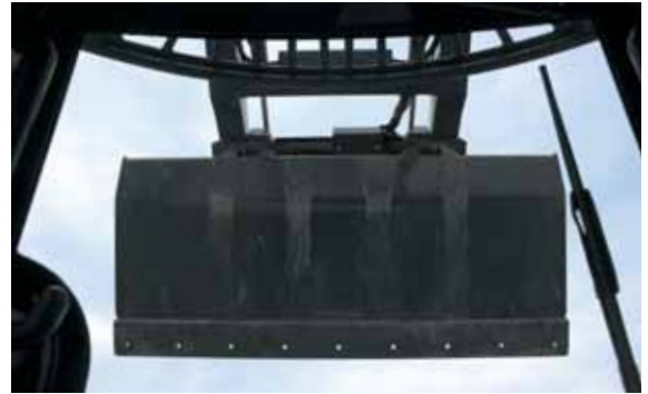
The see-through area on the cab roof provides a clear view to the bucket or attachment, even when it's positioned at full height.
